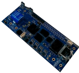
SHM300 Mezzanine-based Tier 3+ SOSA chassis manager
