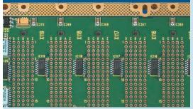
In this case, the option for automatic daisy chaining is achieved due to an "or" logic integrated onto the backplane. When the daughterboard is extracted, the logic closes the daisy chain.
