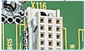
Due to the use of connectors with integral mechanical switches, the contact is automatically opened when the daughterboard is inserted, and closed again when it is extracted.
