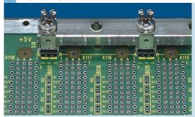
Infeed of the main operating voltage + 5 V/+ 3.3 V and GND is achieved via busbars with an M6 screw connection. The auxiliary operating voltages are supplied via double-FASTONs with an additional M4 screw terminal. The arrangement of the feed modules on the backplane ensures optimum power supply to the daughterboards for problem-free operation.
