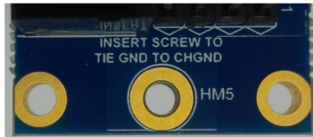
Figure 3-1: Digital Ground – Chassis Ground Tie Point
