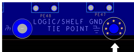
Figure 3-1: Digital Ground – Chassis Ground Tie Point
