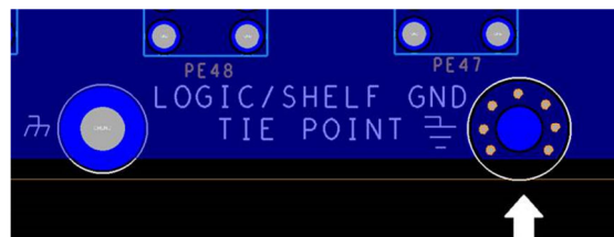
Figure 3-1: Digital Ground – Chassis Ground Tie Point
