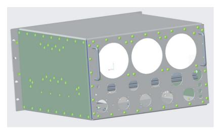
Drawing of Example #2 (Front to Rear Airflow, Recessed, SOSA Aligned)
