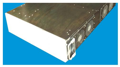
This 3U tall rugged chassis features horizontal loading for 6U, 3U, or a 3U/6U hybrid approach for OpenVPX boards. The cooling is side to side. The boards can be recessed inside the chassis with provisions for MIL 461 for EMI.
