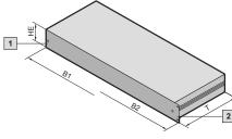
Material/surface finish: Side panels: Extruded aluminium section, untreated Base/cover trays: Aluminium, clear-chromated Front/rear panel: Extruded aluminium section, clear-chromated Mounting plate: Sheet steel
