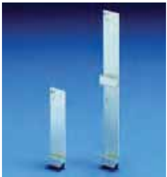
Flat front panels with type V handle and PCB holder Complete modular systems Material: Front panel: 2.5 mm aluminium, natural anodised Handle: aluminium, natural anodised PCB holder: polycarbonate Supply includes: 1 front panel, 1 handle (2 with 6 U), 1 PCB holder (2 with 6 U), assembly parts.
