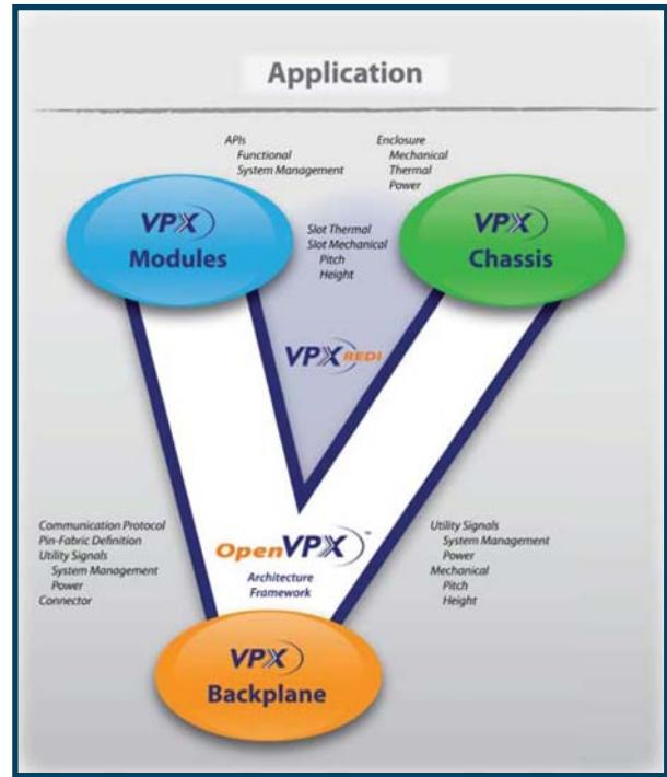
OpenVPX defines clear interoperability points necessary for integration between Module to Module, Module to Backplane and Chassis. The OpenVPX V1.0 Specification, developed by VITA members, has been turned over to the VSO in October 2009 as VITA 65 for final comment, ballot, and ratification as a standard.
