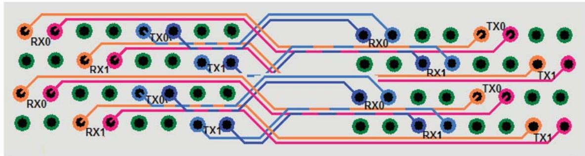
**Thin Pipe:** A channel comprised of two links (2 Tx pairs + 2 Rx pairs). 5Gbps capable 10/100/1000Base-T, 1000Base-BX, PCIe-x2, sRIO-x2, Infiniband-x2
