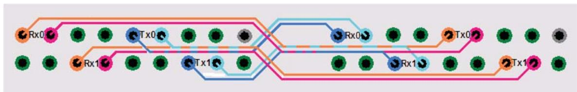
**Ultra-thin Pipe:** A channel comprised of one link (1 Tx pair + 1 Rx pair). 10GBase-KR, 1GBase-KX, PCIe-x1, sRIO-x1, Infiniband-x1a
