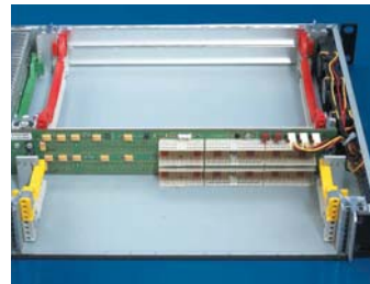
Monolithic cPCI Backplane with H.110 bus (from 2U).
