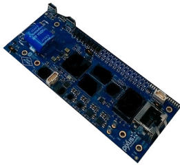
SHM300 Mezzanine-based Tier 3+ SOSA chassis manager
