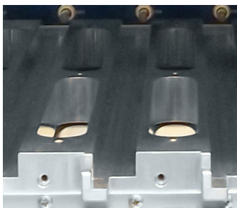
VITA 48.5/48.9 Air Flow Through (AFT) Designs
