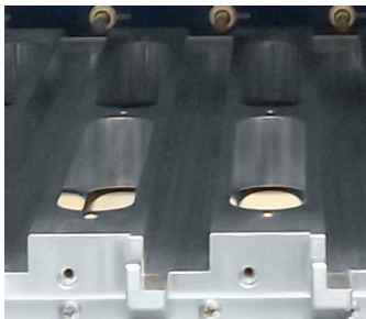
VITA 48.8 Air Flow Through Module Card Guide Tray
