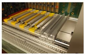
The conduction-cooled card guides allow modules with wedge locks to be plugged into the enclosure.
