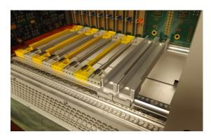
The conduction-cooled card guides allow modules with wedge locks to be plugged into the enclosure.
