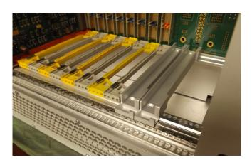
The conduction-cooled card guides allow modules with wedge locks to be plugged into the enclosure. This is used only for prototyping and development.
