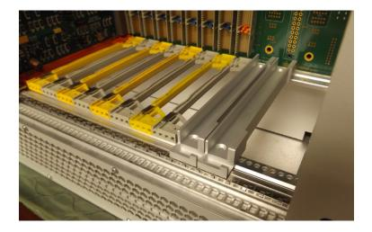
Optional conduction-cooled card guides allow modules with wedge locks to be plugged into the enclosure.
