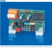
The filter module serves to suppress interference on the + 12 V power supply. In addition, a signal is generated in the event of a fan failure or a significant drop below the nominal speed (displayed via the LED display board).
