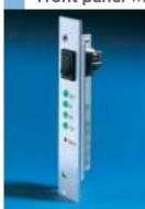
Front panel with switch module and display board with LEDs.
