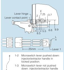
Suitable for CompactPCI and other hot swap applications using a front panel injector/extractor handle operated device.
