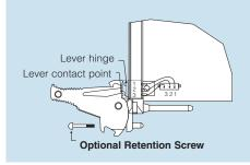
Front panels with injector/extractor handles may retain the pluggable boards in the system by only using the self-locking feature of the handle or by using retention screws.
